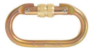
← → Means the major axis gate closed and locked, 25kN means loading rate; HOATER means brand name and HT-R02 means model number;
